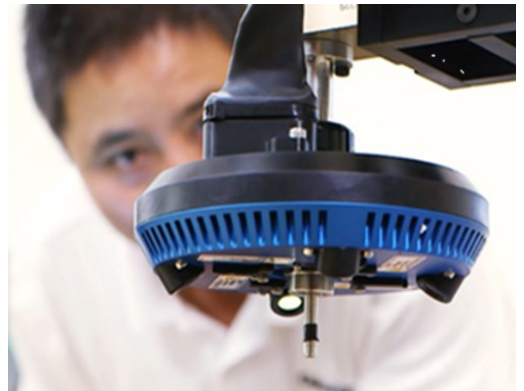
A 3D sensor is mounted around a dispensing nozzle for a 360° view.
