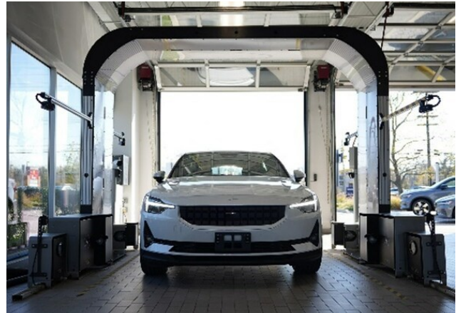
High-speed UVEye vehicle inspections take seconds to complete.
