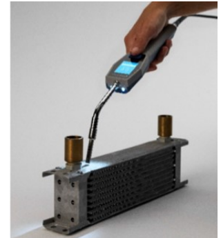
Leak testing soldered oil-cooler connections
